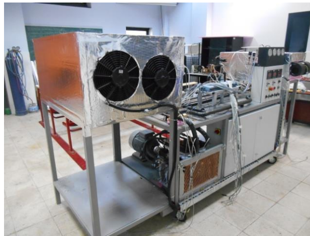
Figure 2. Photograph of the experimental AAC/AHP system.
